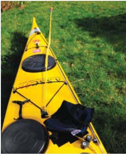
Deck tow deployed. The line is daisy-chained for a short tow, but can be lengthened for a longer distance.
